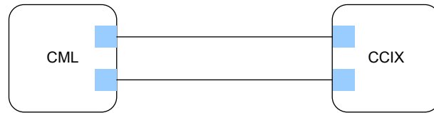
2-socket system with Port Aggregation
